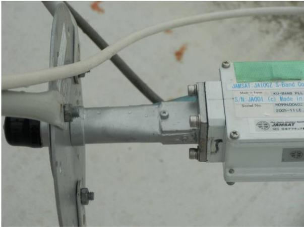
LNB 10.4GHz, Horn Feed,
