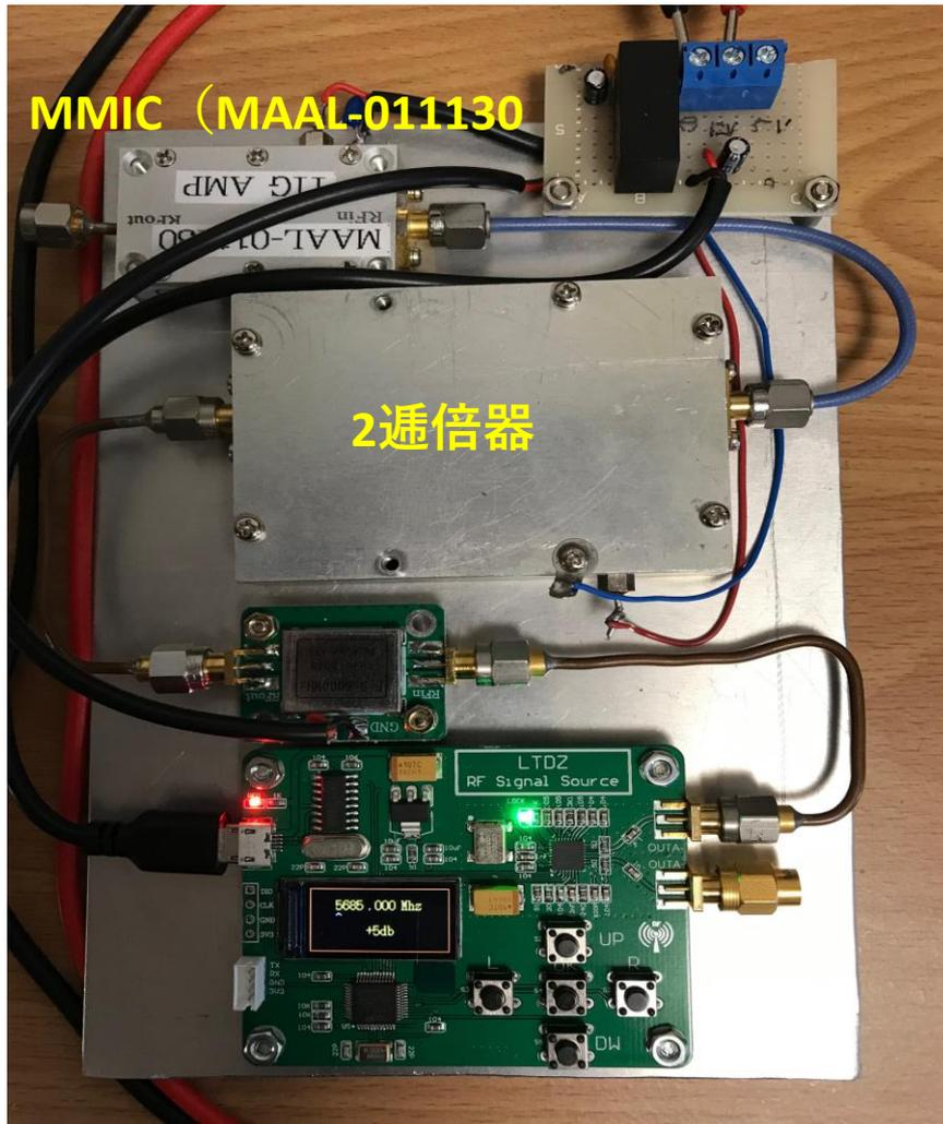
MAX2870 23.5-6000MHz RF Signal Source Generator
