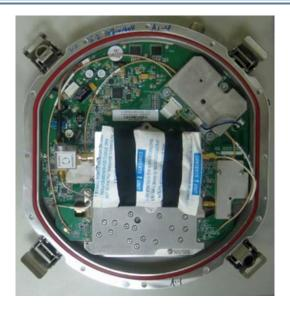
During last periode of time, parts from scrapped Wavelab ODU SP+ are available on Ebay. Most common ODUs are designed for 18GHz, 23GHz, 38GHz. 23GHz item has been studied in detail by our Polish colleagues. Wavelab topic can be found on **Mikrofale**.Cafe forum. RF unit can be easily reused to 24GHz with excellent results (2W maximum output).
